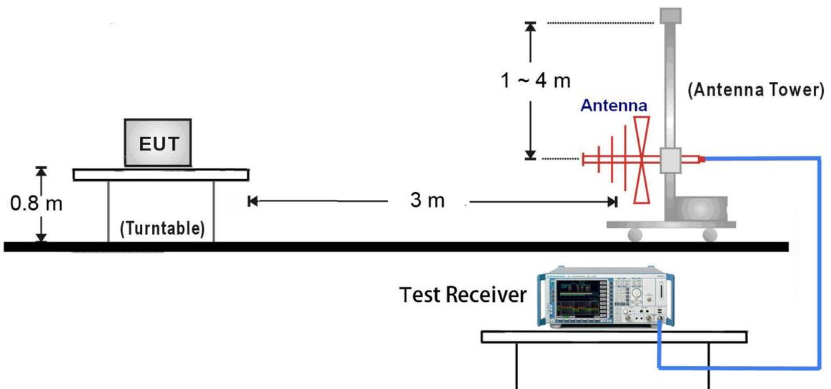
1GHz ~ 18GHz Test Setup:
