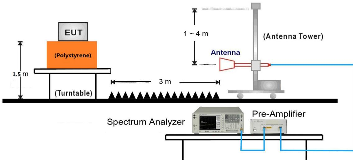
18GHz ~25GHz Test Setup:
