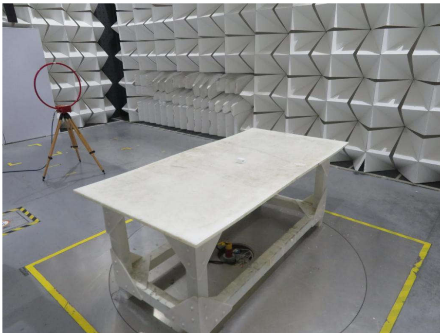
Radiated spurious emission Test Setup-1(Below 30MHz)
