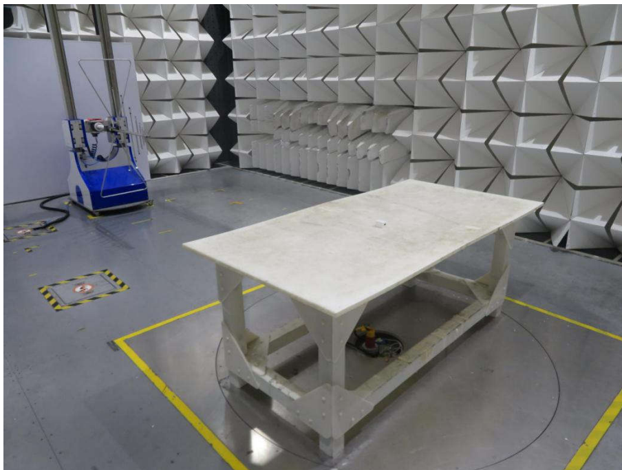
Radiated spurious emission Test Setup-2(30MHz-1GHz)
