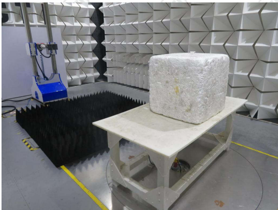
Radiated spurious emission Test Setup-3(Above 1GHz)
