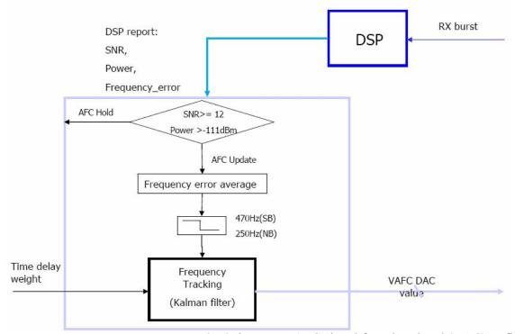
In MT6572, it uses an AFC signal from baseband (DAC) to finish automatic frequency control.
