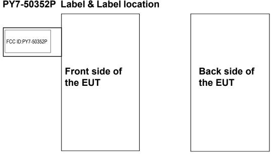
The FCC ID is not on the exterior of the device but labelling meets the conditions allowed in KDB 784748 for the label to be placed in a user accessible area:
