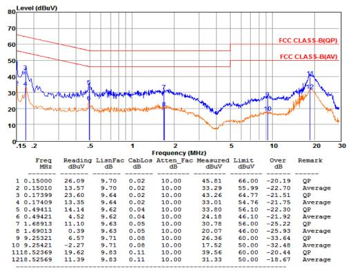
Remarks: 1. Measured = Reading + Lisn Factor +Cable Loss+Atten\_Fac.
