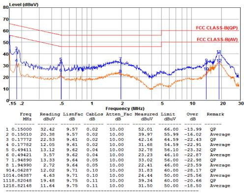
Remarks: 1. Measured = Reading + Lisn Factor +Cable Loss+Atten\_Fac. 2. The emission levels that are 20dB below the official
