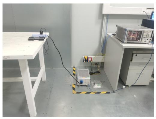
Radiated emission test 30MHz – 1GHz
