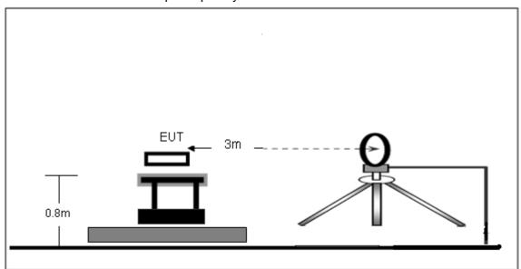
(B) Radiated Emission Test-Up Frequency 30MHz~1GHz
