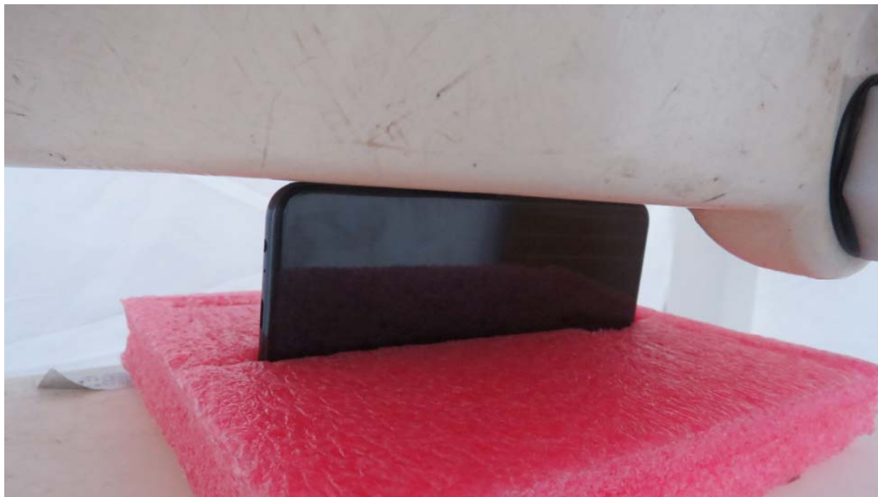
Picture 13: Left Side, the distance from handset to the bottom of the Phantom is 0mm
