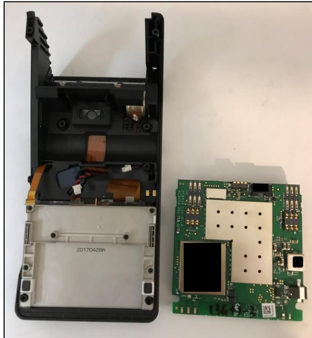
Top Cover & PCB- Top View
