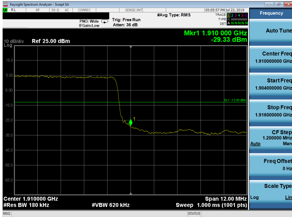
Plot 7-154. Upper Band Edge Plot (Band 2 - 15.0MHz QPSK - Full RB Configuration)
