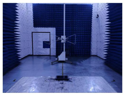
RADIATED EMISSION TEST SETUP ABOVE 1GHz- P01V71
