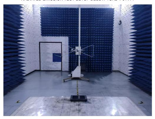
RADIATED EMISSION TEST SETUP BELOW 1GHz- P701
