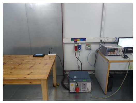
RADIATED EMISSION TEST SETUP ABOVE 1GHz- P701
