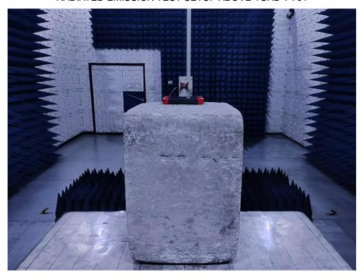
RADIATED EMISSION TEST SETUP ABOVE 1GHz- P711
