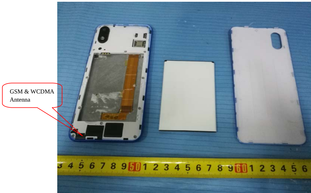
EUT – Cover off View 1
