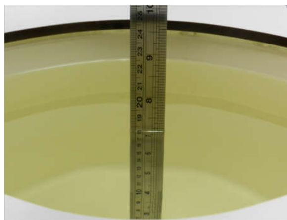
Fig 10.2 Photo of Liquid Height for Body SAR
