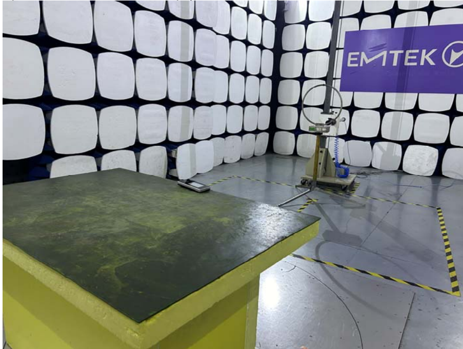
Spurious Emission Test Setup (Below 30MHz)
