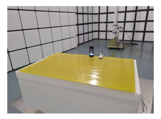
**Photo of Radiated Emission Measurement (Above 1GHz)**
