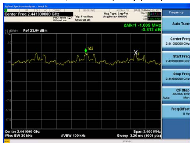
BT 3DH5 CH39, Carrier frequency (MHz): 2441
