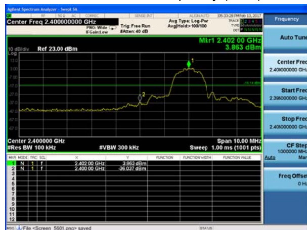
BT 3DH5 CH0, Carrier frequency (MHz): 2402
