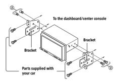
When mounting this unit to the preinstalled brackets of your car, use the supplied screws ② in the appropriate screw holes based on your car: T for TOYOTA and N for NISSAN.
