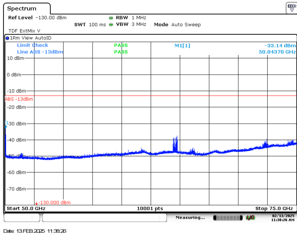
Figure 8.5-24: Radiated emissions spectral plot (50 GHz - 75 GHz) high channel vertical
