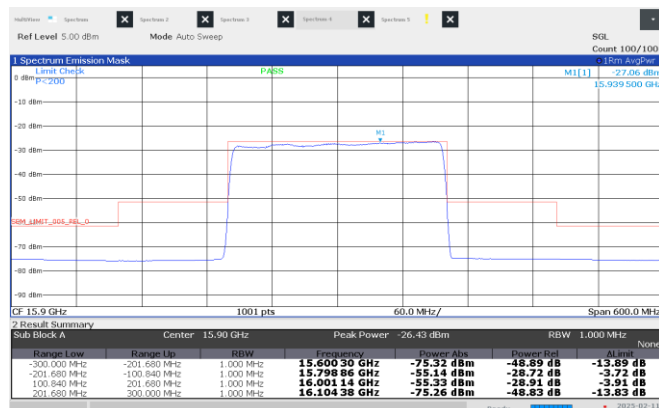
Figure 8.4-65: Emission mask, Low channel: 15.90 GHz, shortest pulse. (200 MHz BW)
