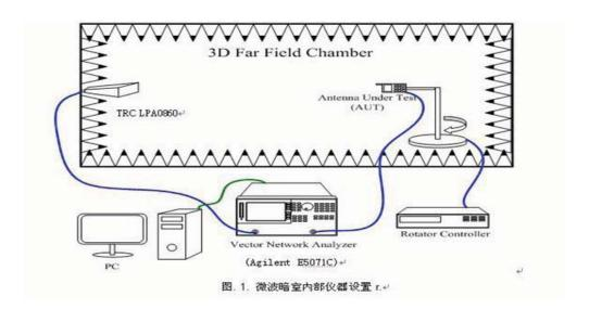
Figure 1 shows the instrument settings and network analyzer connection diagram in the microwave darkroom. The distance from the transmitting antenna (the transmitting antenna model used in this darkroom is TRC LPA0860 800MHZ-6GHZ) to the antenna under test (AUT) is 1.35 meters. The antenna under test is placed on a rotating platform. By controlling the rotation angle of the turntable, the antenna under test can be roughly and more accurately measured.
