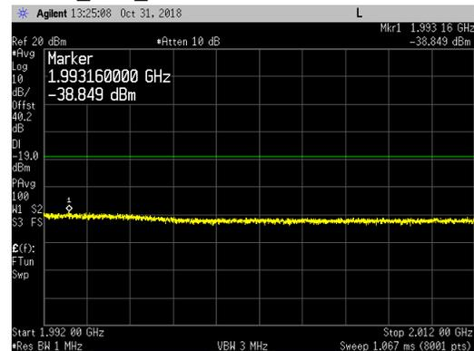
**Band 2 Single Carrier at Reduced Power -Lower and Upper Band Edge Plots:**
