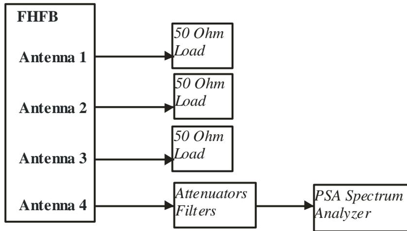
Test Setup Used for FHFB Conducted RF Measurements
