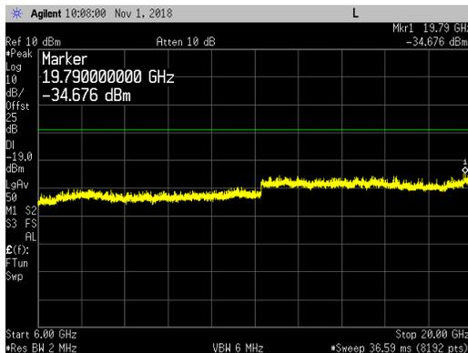
**Three Multiradio Carriers at Max Port Power (40W) \_GMSK at 1930.4 & 1965.0MHz, LTE5 at 1933.3MHz:**
