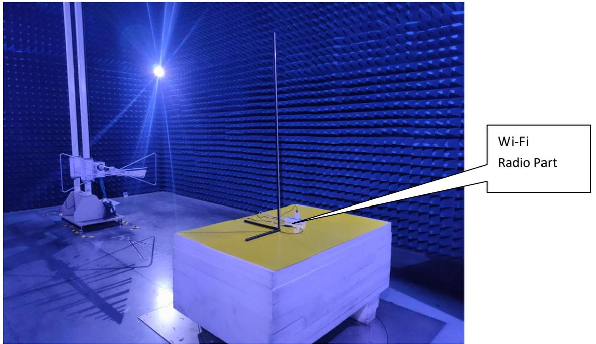
Photo of Radiated Emission Measurement (Above 1G)
