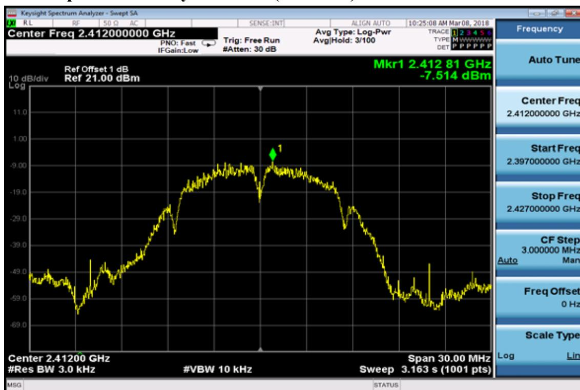
**Power Spectral Density Test Plot (CH-Mid)**
