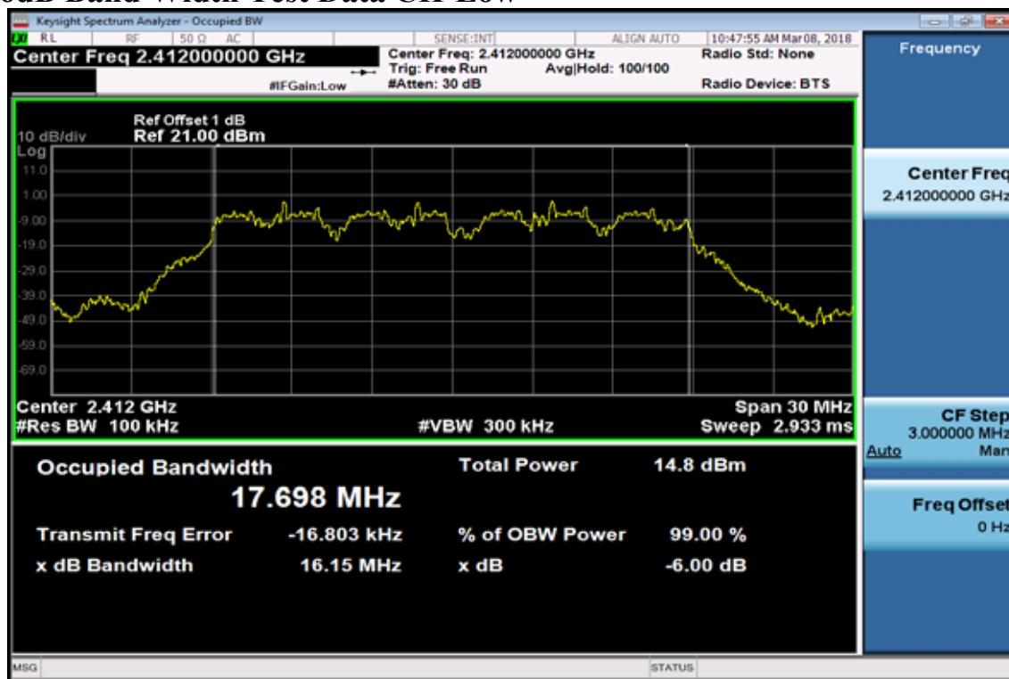
**6dB Band Width Test Data CH-Mid**
