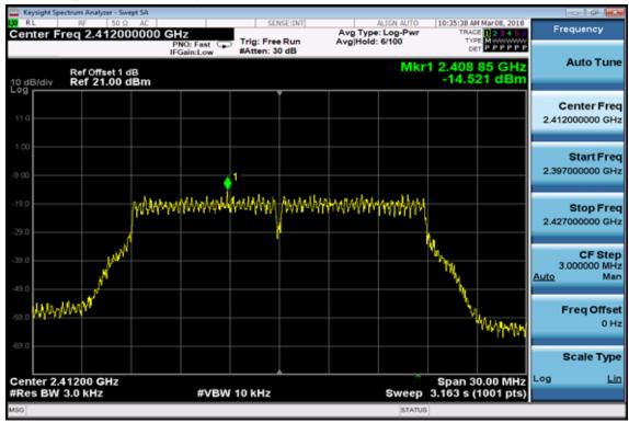
**Power Spectral Density Test Plot (CH-Mid)**
