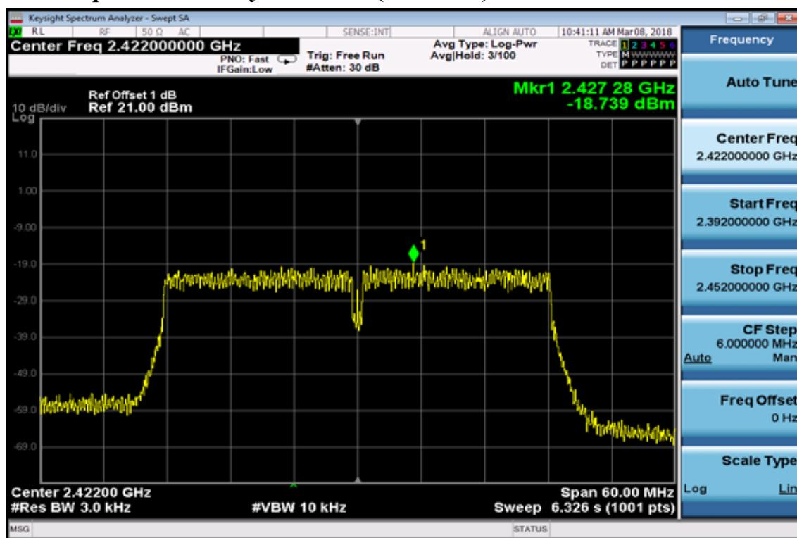
**Power Spectral Density Test Plot (CH-Mid)**
