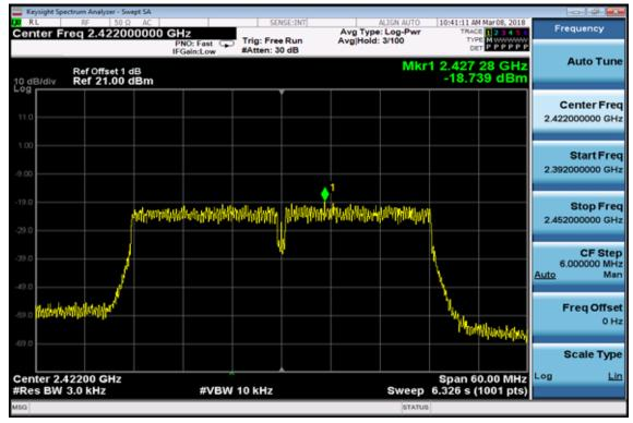
Power Spectral Density Test Plot (CH-Mid)
