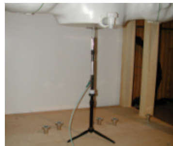
Figure 12.1 Dipole Validation Test Setup
