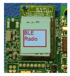
The left picture is the original module that was certified. The picture on the right is the module implemented in the new end-product. Antenna is on the module and therefore was not modified when installed on host board.
