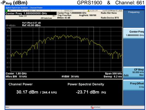
PAPR (dB) =  $P_{Pk}$  (dBm) -  $P_{Avg}$  (dBm) = 30.31 dBm - 30.17 dBm = 0.14 dB
