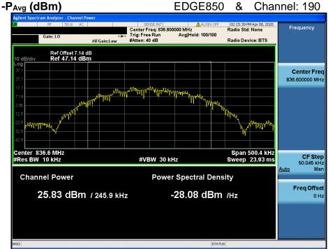
$PAPR (dB) = P_{Pk} (dBm) - P_{Avg} (dBm) = 29.28 dBm - 25.83 dBm = 3.45 dB$
