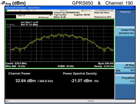
$PAPR (dB) = P_{Pk} (dBm) - P_{Avg} (dBm) = 33.07 dBm - 32.84 dBm = 0.23 dB$
