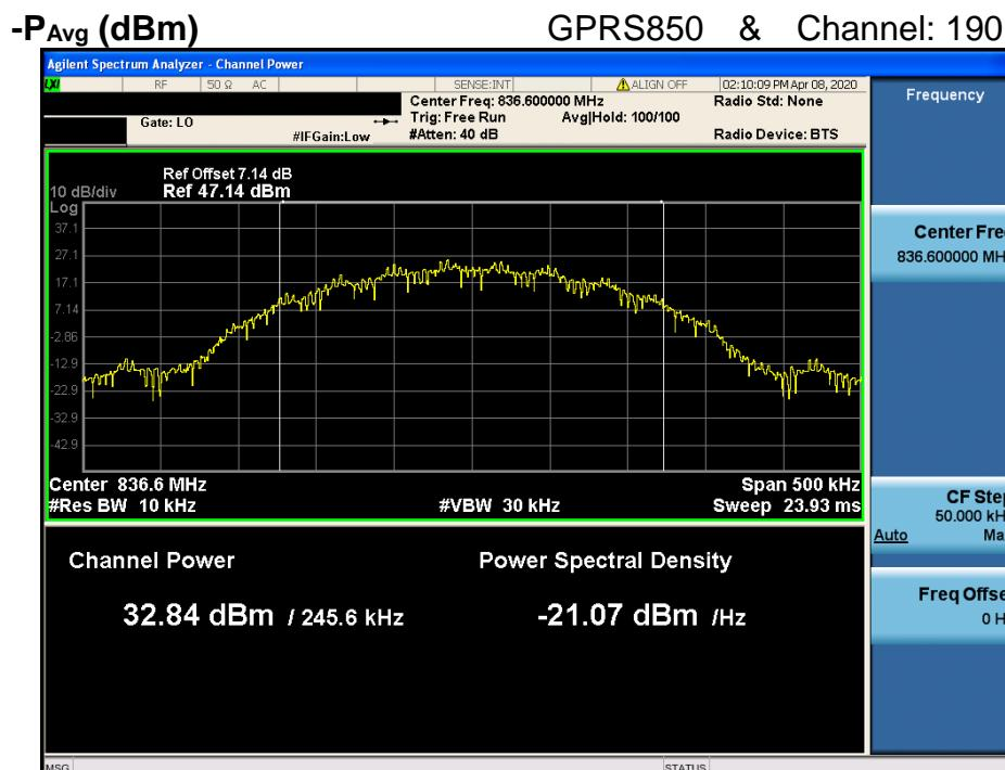
$$\text{PAPR (dB)} = \text{P}_{\text{Pk}} (\text{dBm}) - \text{P}_{\text{Avg}} (\text{dBm}) = 33.07 \text{ dBm} - 32.84 \text{ dBm} = 0.23 \text{ dB}$$
