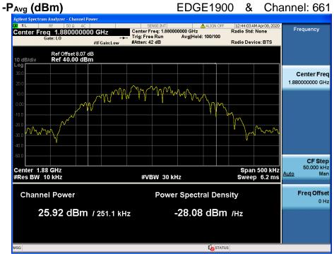
PAPR (dB) =  $P_{Pk}$  (dBm) -  $P_{Avg}$  (dBm) = 29.32 dBm - 25.92 dBm = 3.40 dB
