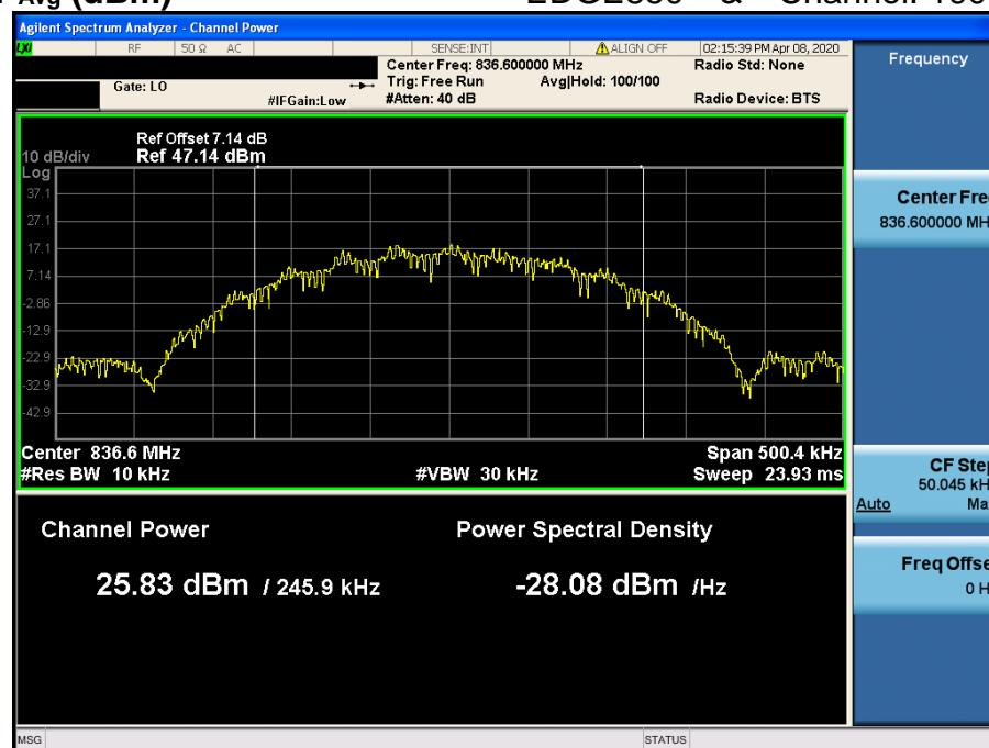
$$\text{PAPR (dB)} = \text{P}_{\text{Pk}} (\text{dBm}) - \text{P}_{\text{Avg}} (\text{dBm}) = 29.28 \text{ dBm} - 25.83 \text{ dBm} = 3.45 \text{ dB}$$
