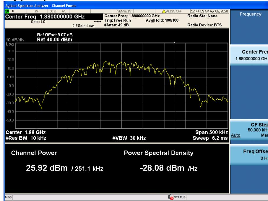
$$\text{PAPR (dB)} = \text{P}_{\text{Pk}} (\text{dBm}) - \text{P}_{\text{Avg}} (\text{dBm}) = 29.32 \text{ dBm} - 25.92 \text{ dBm} = 3.40 \text{ dB}$$
