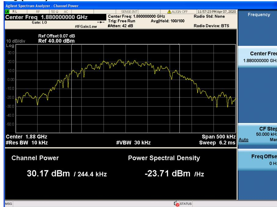
$$\text{PAPR (dB)} = \text{P}_{\text{Pk}} (\text{dBm}) - \text{P}_{\text{Avg}} (\text{dBm}) = 30.31 \text{ dBm} - 30.17 \text{ dBm} = 0.14 \text{ dB}$$
