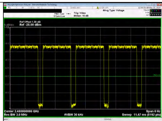
BLE/GFSK 1 Mbps High Channel, 2480 MHz
