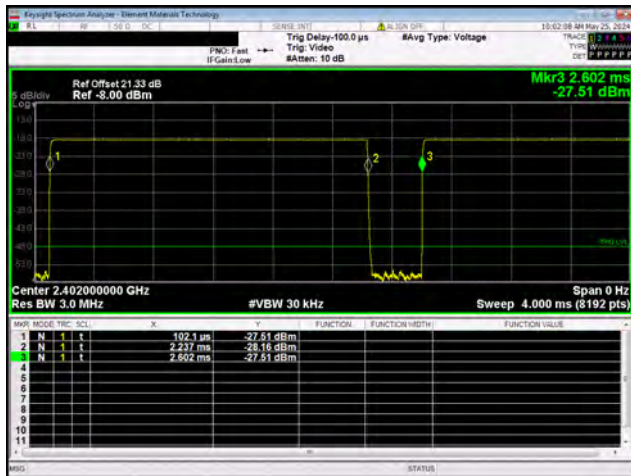
BLE/GFSK 1 Mbps Low Channel, 2402 MHz
