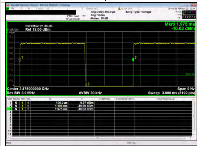
PAS/GFSK 2 Mbps High Channel, 2476 MHz
