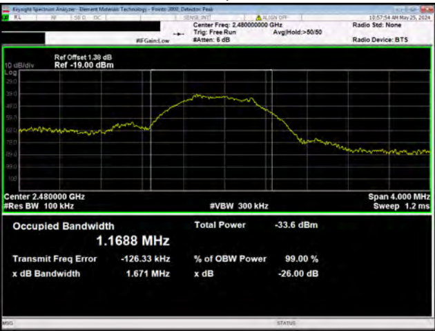
BLE/GFSK 1 Mbps High Channel, 2480 MHz
