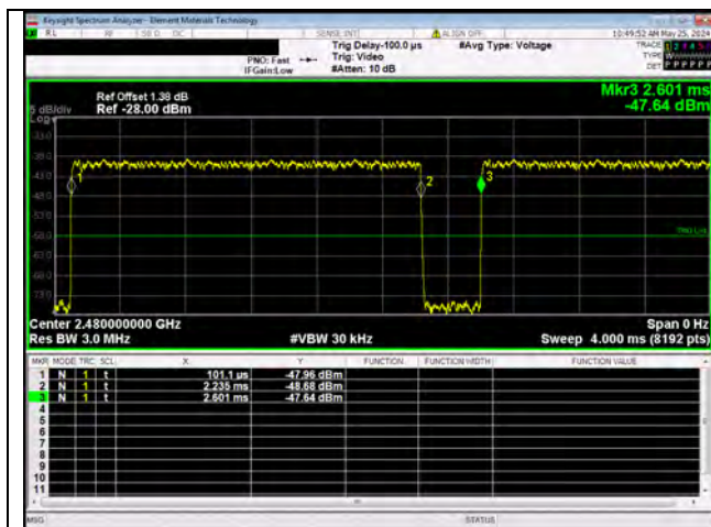
BLE/GFSK 1 Mbps High Channel, 2480 MHz
