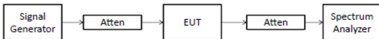
Figure 7.3.1 Out-of-band rejection test setup
