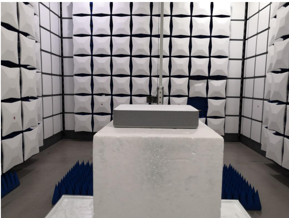
FCC RADIATED EMISSION TEST SETUP ABOVE 1GHZ
