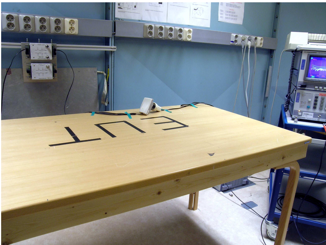
Test setup, Conducted emissions
