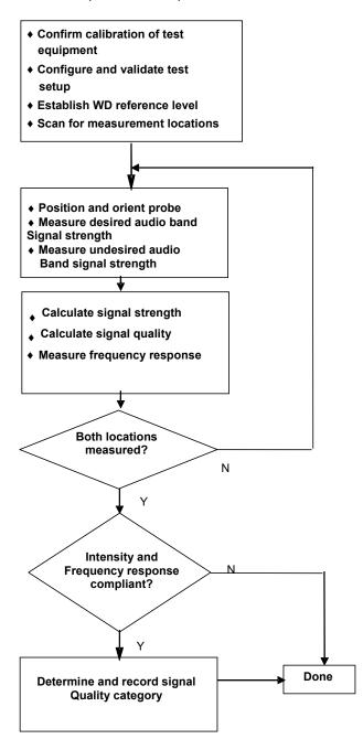
Figure 4-15 C63.19 T-Coil Signal Test Process
