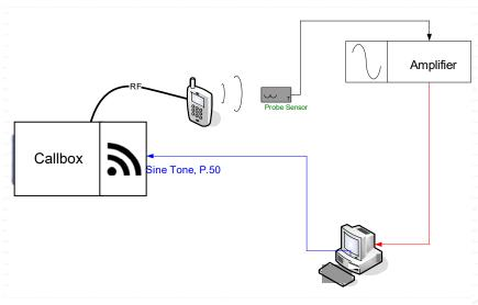
Figure 4-2 T-Coil Test Setup
