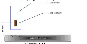
Figure 4-11 Measurement Distance
