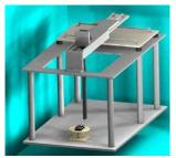
Figure 4-3 RF Near-Field Scanner
