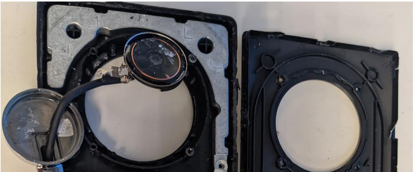
Open enclosure with Antennas Visible
