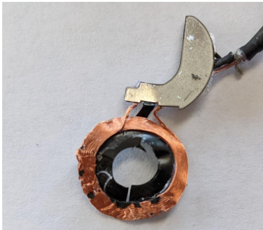
326.5kHz + 1.778 MHz Apple Watch Coil (Bottom)
