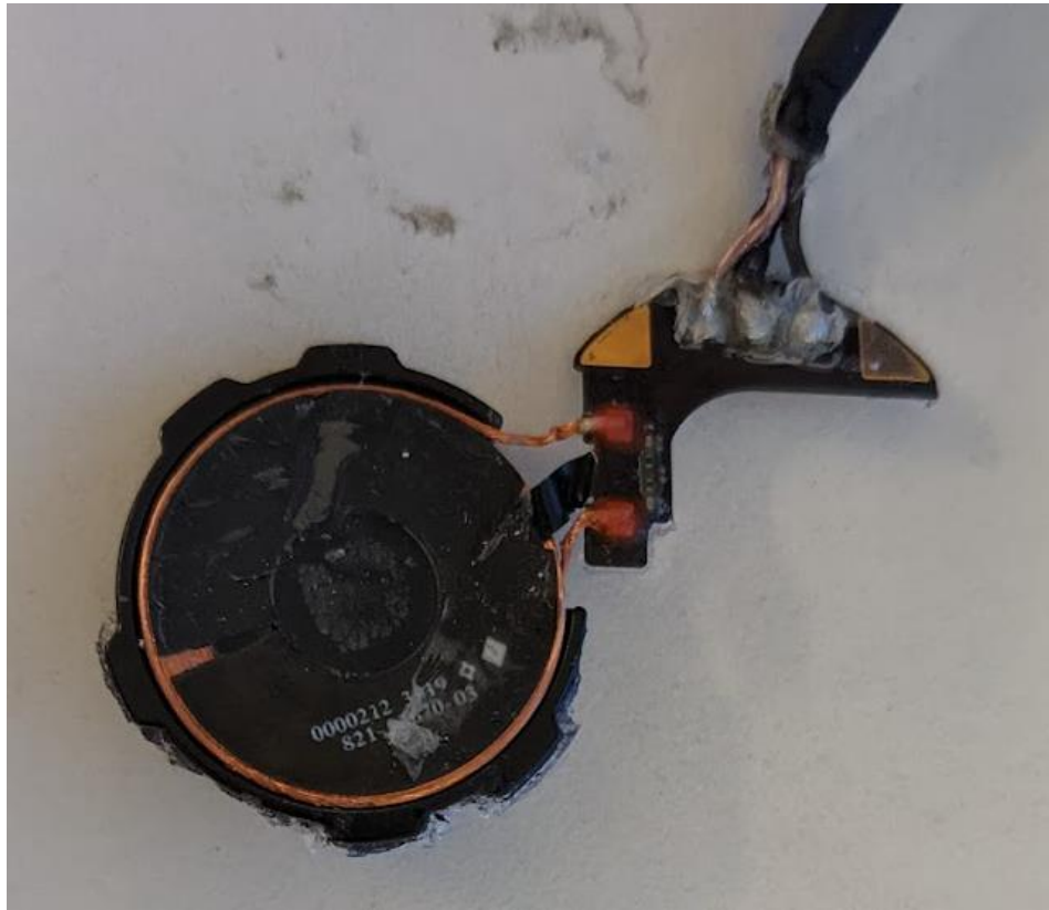
326.5kHz + 1.778 MHz Apple Watch Coil (Bottom)
