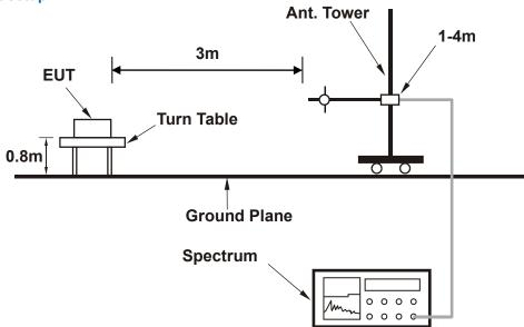
**Note:** For the actual test configuration, please refer to the attached file (Test Setup Photo).the actual test configuration, please refer to the attached file (Test Setup Photo).
