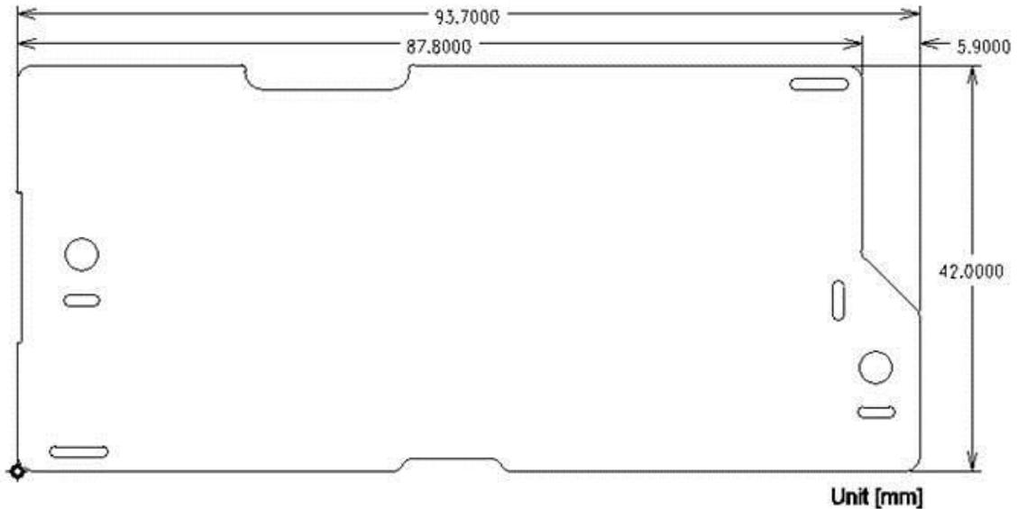
Figure 2. Mechanical dimension
