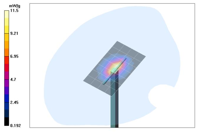
1 g average of 10 measurements: 9.966 mW/g 10 g average of 10 measurements: 5.219 mW/g
