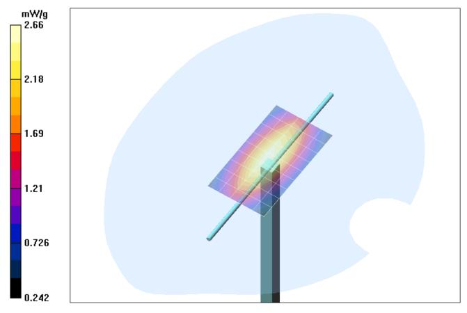
1 g average of 10 measurements: 2.449 mW/g 10 g average of 10 measurements: 1.606 mW/g
