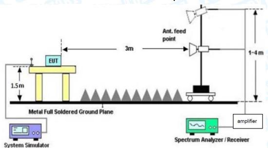
**Above 1GHz Test Setup**
