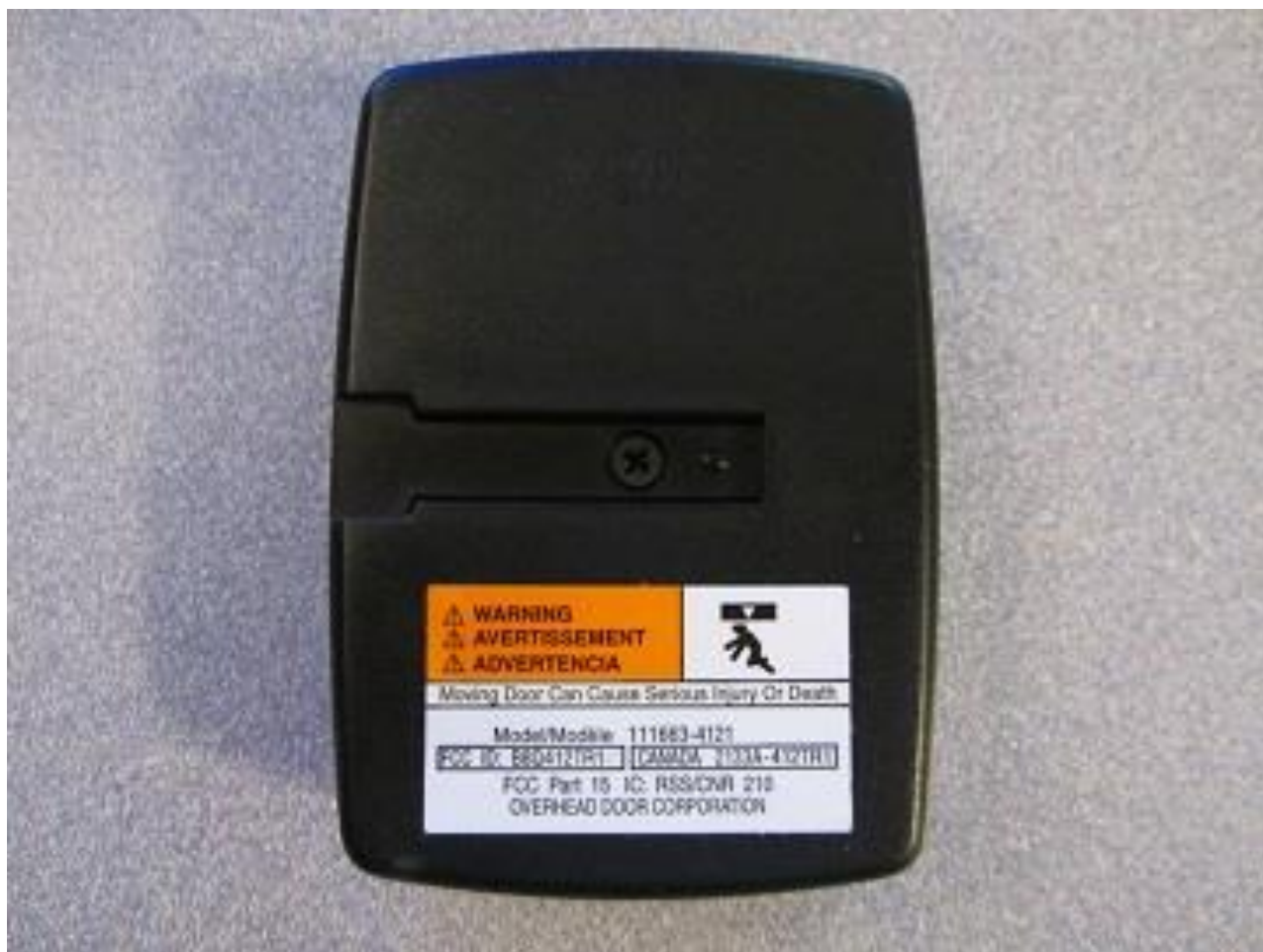
Figure 1: 412TR1 FCC / IC Label Location
