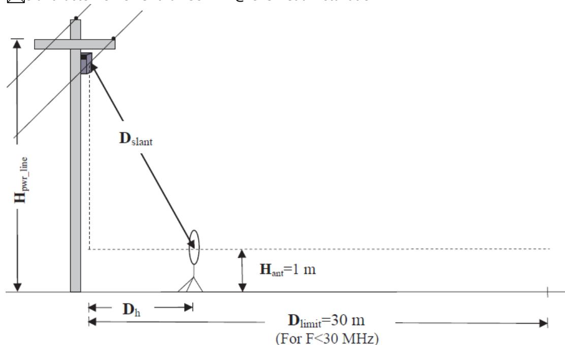
Here  $H_{ant} = 1\text{ m}$ ,  $H_{power\_line} = 2\text{ m}$ ,  $D_h = 3\text{ m}$ ;
