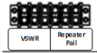
Figure 12; NFPA Dry Contact connection location inside the cabinet
