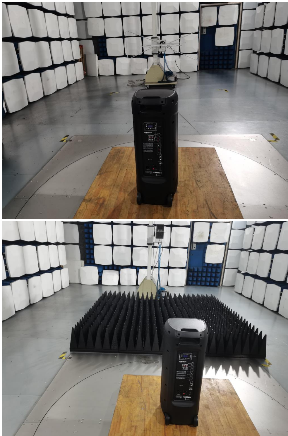
Radiated emission test view
