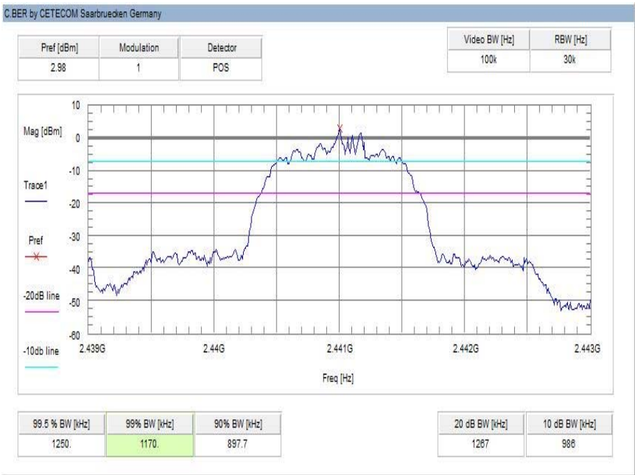
Plot 5: middle channel – 2441 MHz, Pi / DQPSK modulation
