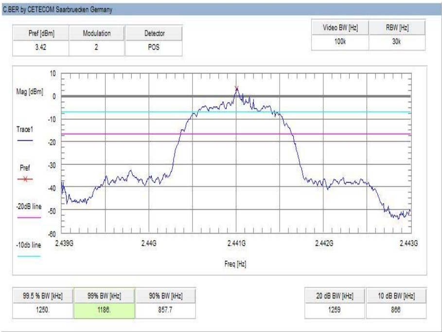
Plot 8: middle channel – 2441 MHz, 8 DPSK modulation
