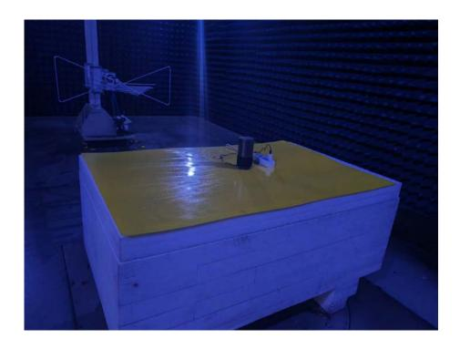
Photo of Radiated Emission Measurement Above 1GHz
