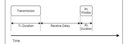
The eDoctor is a LoRaWAN Class A device that is fully compliant with the LoRaWAN Specification v1.0.2 and the LoRaWAN Regional Parameters v1.0.2. These documents specify the Tx and Rx scheme as shown in the figure. These specifications also place limits on the Tx and Rx behaviour as follows:
