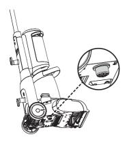
Before each use, clean the casing of humidity sensor, rotate the humidity sensor casing 3 times clockwise and counterclockwise respectively.
