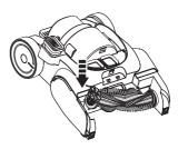
Replace the brush roller by inserting the brush roller end into the right side of the holder, then attach the roller tab to the left side to lock into place.
