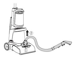
Press the buttons on both sides to remove the hose.
