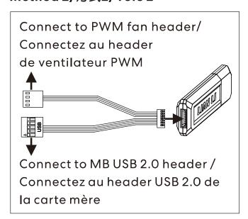
Each L-Wireless Controller supports 10 channel of device/
