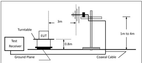
(c) For radiated emissions above 1000MHz
