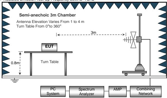
(C) Radiated Emission Test-Up Frequency Above 1GHz
