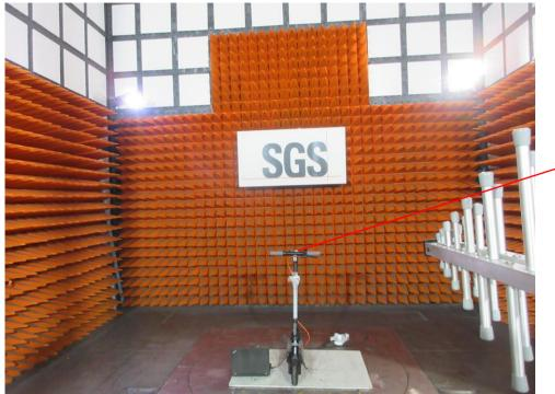
RF antenna and module are located in the handle at above 0.8m from the floor.
