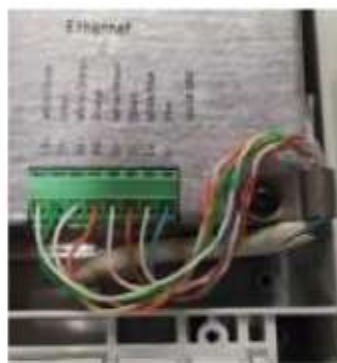
Figure 15: Detail of the connections for the Power through PoE.
