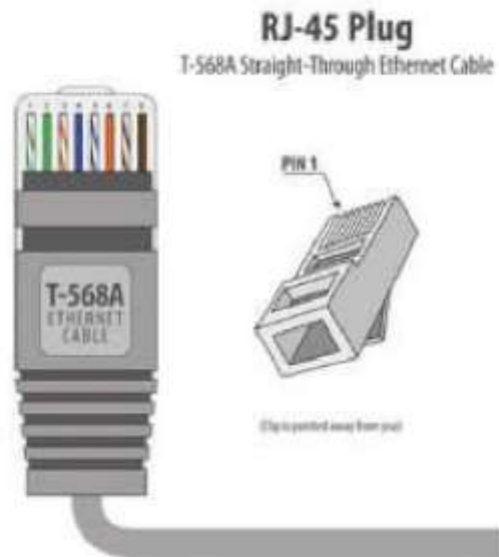
Figure 17: Wiring of the cable at the RJ45 connector (following T-568A/B specification) to be inserted in the PoE injector.
