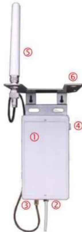
Figure 13: LS-G6 Gateway, with all the parts indicated.
