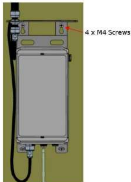
Figure 20: Gateway mounted on the wall.
