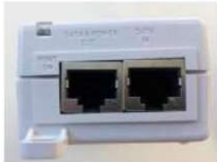
Figure 26: PoE. Left port (Data & Power Out) is for the power cable and right port (Data In) is for data transmission.
