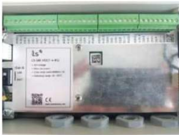
Figure 48: View of the LS-G6-ANALOG datalogger internally where the four channels can be identified.
