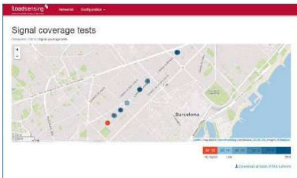
Figure 51: View of the geographical display (in the software of the gateway) indicating the results of the signal coverage tests.
