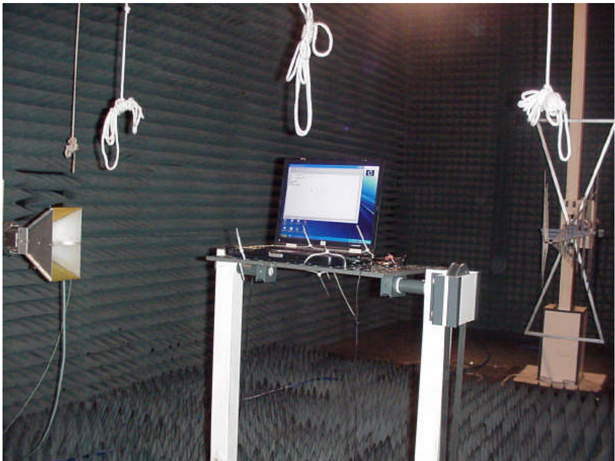
Photo 3: Setup for radiated measurements (EUT in the laptop)
