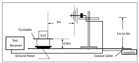
(c) For radiated emissions above 1000MHz
